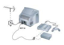
Carry out the connections as shown. 2 To optimise picture quality, connect the equipment which produces the video signals (digital decoder, games, etc) to AV1 in and equipment which produces the S-Video signals S-Video and Hi-8 video recorders, certain DVD drives to AV2 in and all other equipment to either AV1 in or AV2 in.
